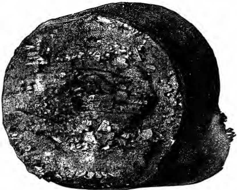
FIG. 90.—FRACTURED SURFACE OF CONNECTING ROD.
